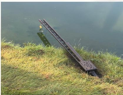
We have two areas that we have had installed the new lake monitoring system. We have been adjusting the sensors and believe that we have it dialed in. Now we watch and see!! The sensors will be pulled from the water when the fountains and circulator pump are removed for the winter season. As you can see in the picture, the black metal will remain all winter season, only the small sensors at the end will be retracted for the winter.
